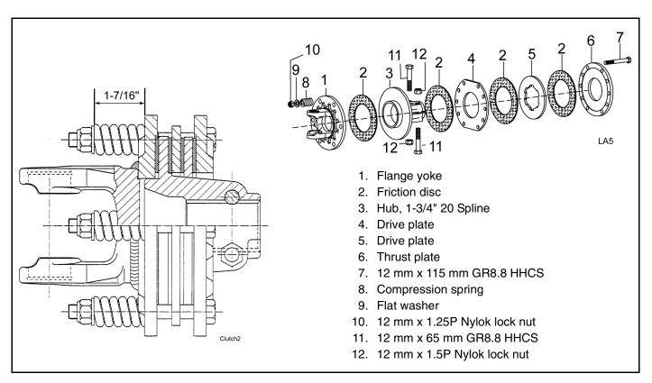
Figure 12. Slip Clutch Assembly
